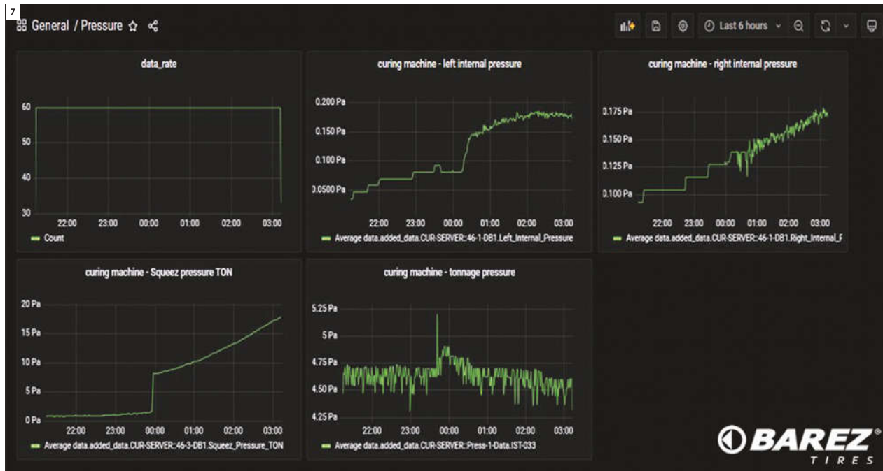
Figure 7: Dashboard of tire curing press pressure developed for the Barez Industrial Group
